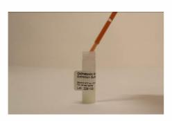
1a. Add 1 ml of wine to an extraction vial. Close the vial and shake well for 1 min.
