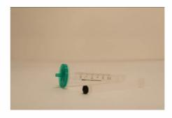
2a. Remove a plunger from a syringe and attach a filter to the syringe.
