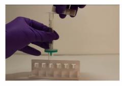
3a. Mix the content of the extraction vial and pour quickly into the syringe.
