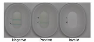
If the sample is negative for OTA (<1  $\mu$ g/l) then two blue coloured lines appear (C + T). If the sample is positive for OTA (≥1  $\mu$ g/l) then only one blue coloured line (control line) appears (C). The test is invalid when no blue coloured line appears. The sample should be retested.
