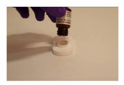
6. Pour the content of the extraction vial onto a FTR device. Allow the liquid to flow-through completely.
