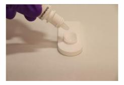
8b. Add 3 drops of substrate onto the device.
