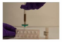
4a. Attach the plunger and filter the sample into a clean sample tube/container. The filtrate is now ready to use.
